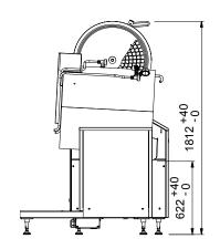
CWI1 Cold Water inlet 1 (cleaning) Electrical inlet (power) Hot water inlet HWI
